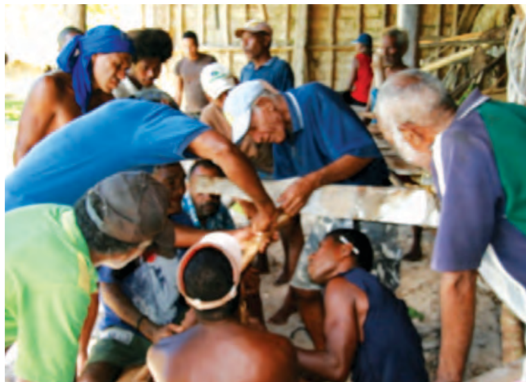
It takes a village to build a voyaging canoe. Many of the complex lashings that hold the vessel together require more than one pair of hands to create.
