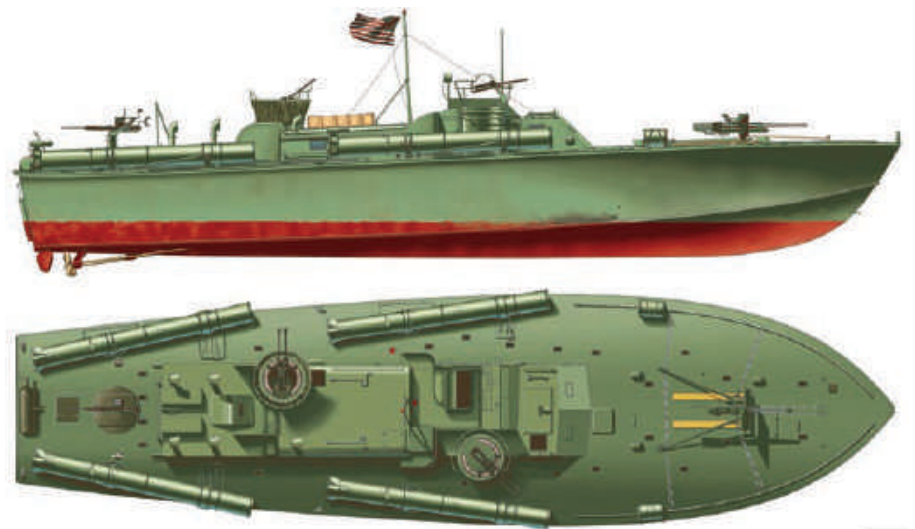
Top right: A US motor torpedo boat similar to the PT109 which split in two during the skirmish off Gizo. Right: A side and aerial view of the boat, which was made from wood and steel and could travel at speeds of up to 41 knots. Photos: Naval Historical Center
